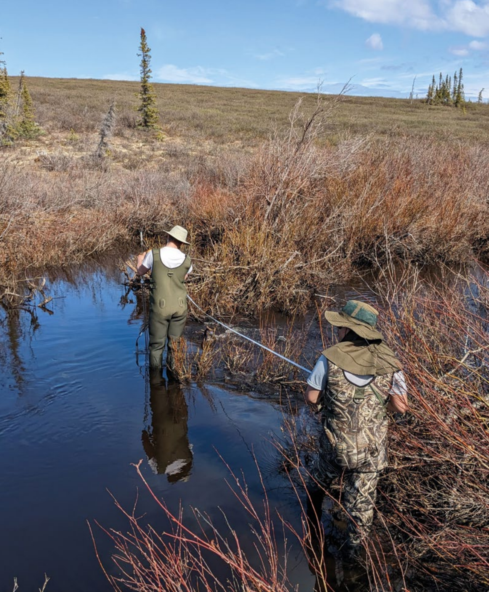
PHOTO: ALEXANDER FOGAL, Wilfrid Laurier University For historic purposes, as well as many ongoing projects, measuring stream flow is a critical component. Pictured is Malcolm Brockett, measuring stream flow at set points along the cross section of the stream, and Jackson Seto holding the measuring tape.
